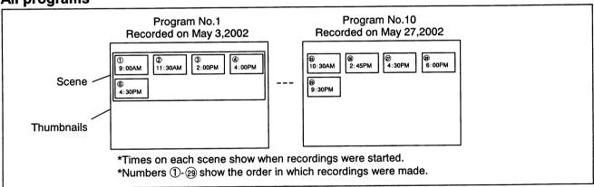
Scenes of one program are lined up in the order of recording. Usually, when the button is pressed immediately after recording, the last scene of the last program on disc (scene a of program No. 10 in the above diagram) will be played back.
